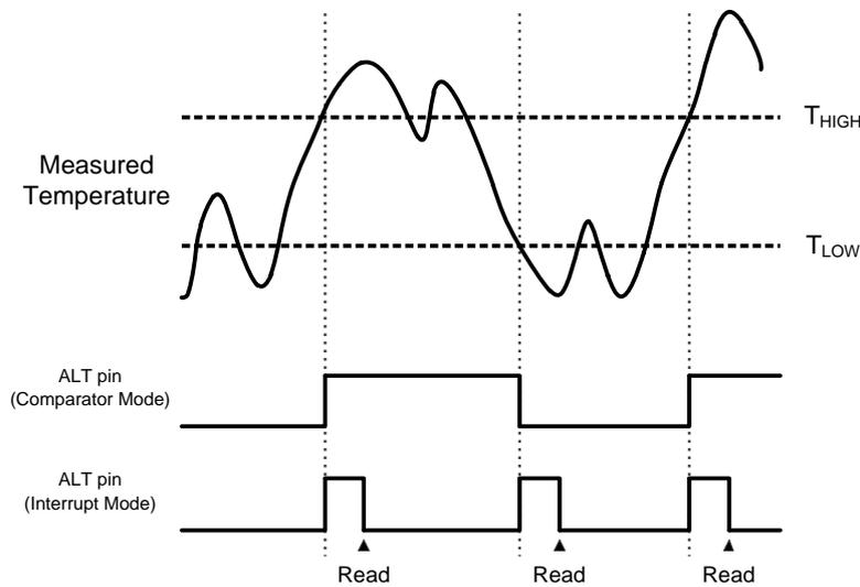
Figure 2. ALT Pin Modes of Operation
