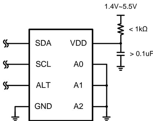
Figure 6. Typical Connections of the GD30TS076C
